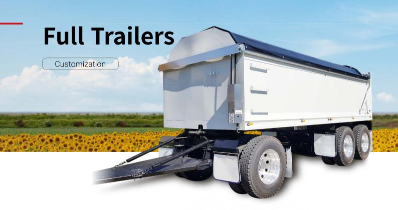
Tow truck as a trailer that has a structure capable of having the entire weight of the truck itself and the freight absorbed by its front and rear axles only.
